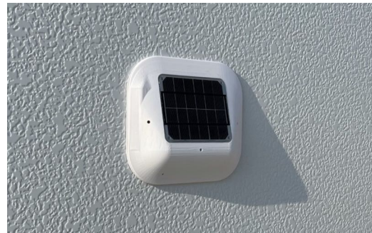
Figure 2. Mote mounted on a wall with magnets.
