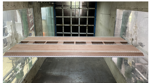
(a) Center-slotted girder model with regularly-arranged grids
