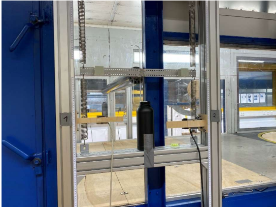
Figure 2. Wind tunnel tests on an elastically suspended circular cylinder.
