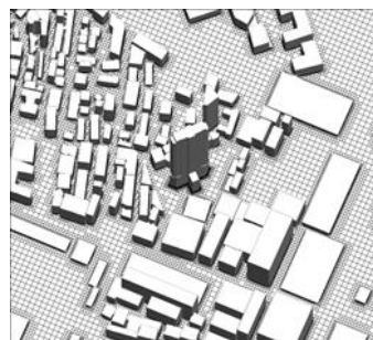
Figure 5. Mesh refinement around building blocks
